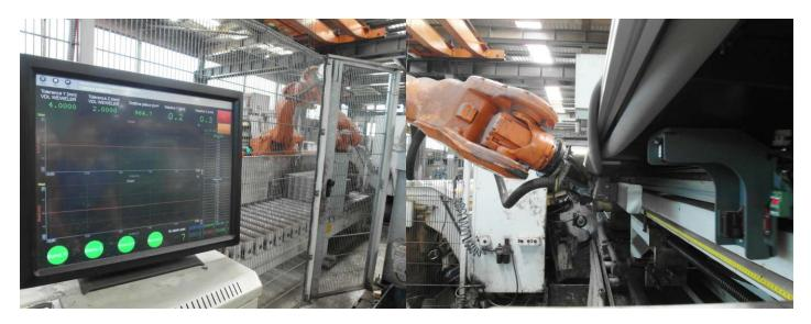
Flat steel is sold in rolled length and according to customer's demands in shorter lengths as well. It is cut in the Rolling Mill on shears and band saw and in the Cold Finishing on circular saws with robotic bundling of cut bars.
